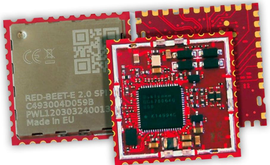
Figure 1: RED-BEET-E 2.0 for electric vehicle supply equipment (EVSE).
