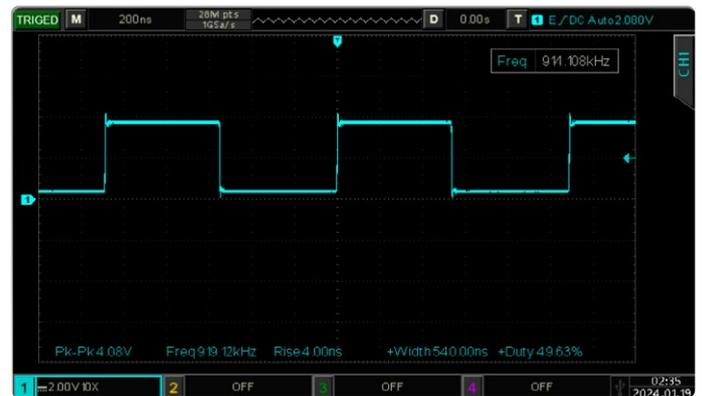
Figure 3: ESP32-C3-DevKit-M1 generating its maximum frequency while running code compiled by the Arduino framework.
