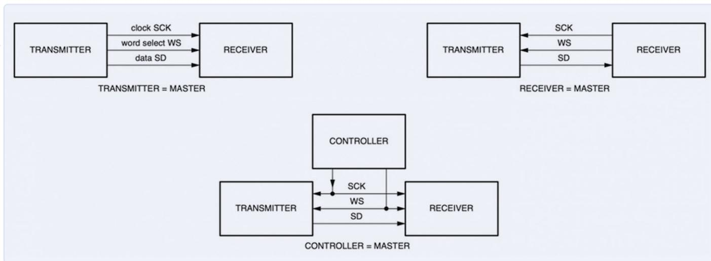
Figure 3: I<sup>2</sup>S configurations (taken from the I<sup>2</sup>S specification).
