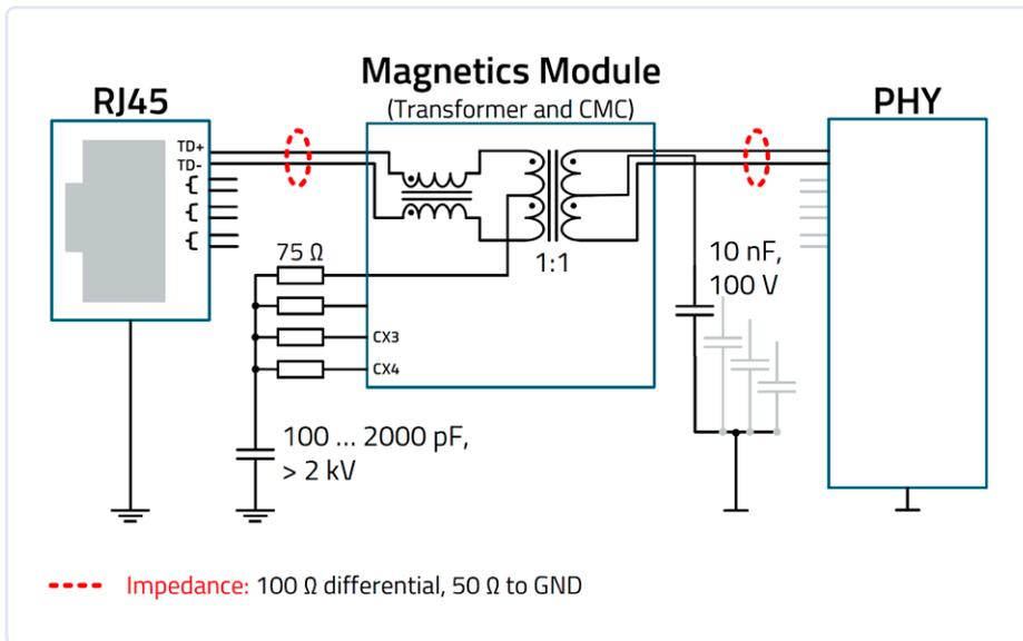
Figure 1: Schematic circuit of a 1 Gbit Ethernet interface. Only one of four channels is shown in the picture. (Source of all images: Würth Elektronik eiSos)
