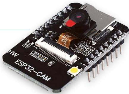
Figure 3: ESP32-CAM module top view.
