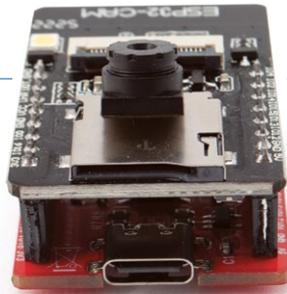
Figure 4: The ESP32-CAM should be inserted in such a way that the socket for the SD card and the USB connector are on the same side.
