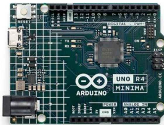
Figure 2: Arduino UNO R4 Minima. (Source: Mouser Electronics)
