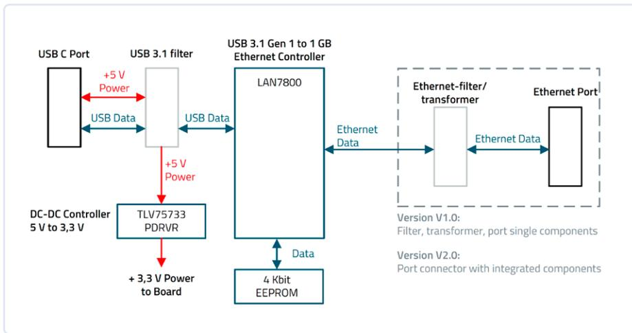
Figure 4: Block diagram of the Gbit-Ethernet-USB adapter board in both versions.
