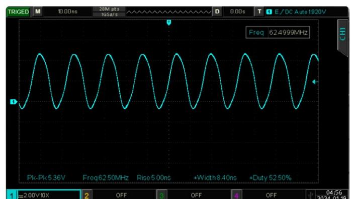
Figure 5: Raspberry Pi Pico W at 62.5 MHz using a PWM function in MicroPython.
