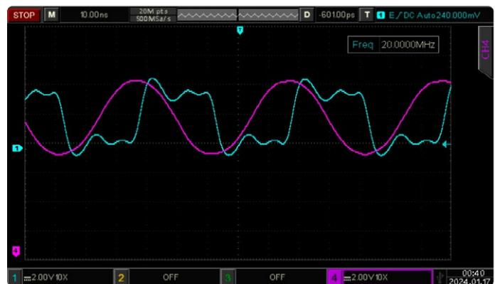
Figure 2: Comparison of square waves between the ESP32-S2 (Blue) and the UNI-T UTG962E (Pink).
