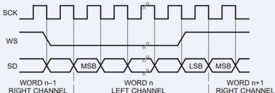
Figure 4: I<sup>2</sup>S bus timing (taken from the I<sup>2</sup>S specification).
