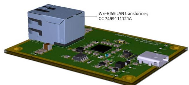
Figure 3: Gigabit Ethernet USB adapter board in the discrete version V2.0: The module with the transformers and common mode chokes is integrated in the RJ45 socket.
