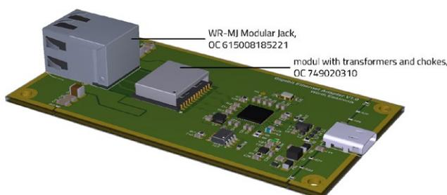
Figure 2: Gigabit Ethernet USB adapter board in the discrete version V1.0: The module with the transformers and common mode chokes is placed next to the RJ45 jack.
