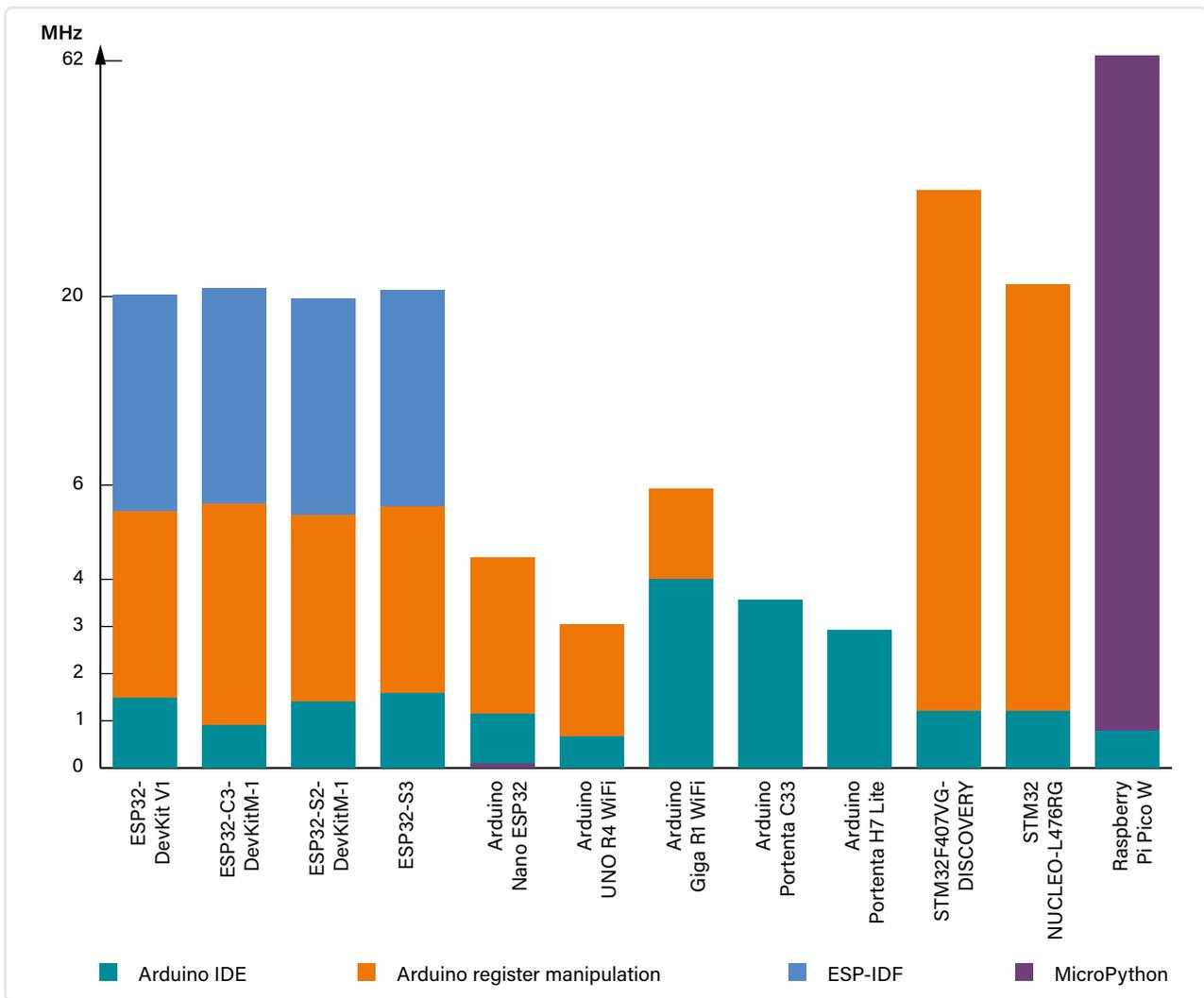
Figure 6: Bar graph showing the maximum output frequencies for the microcontrollers tested.
