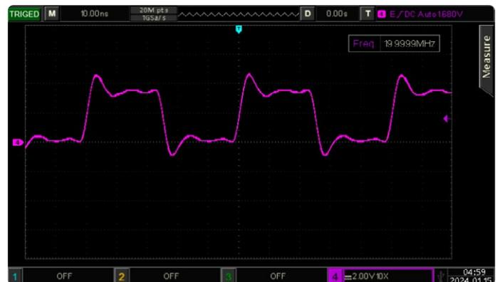
Figure 4: ESP32-C3-DevKit-M1 producing its maximum frequency while running code compiled by ESP-IDF.
