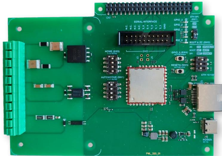
Figure 2: RED-BEET-EVAL-BOARDS for all these types of modules.
