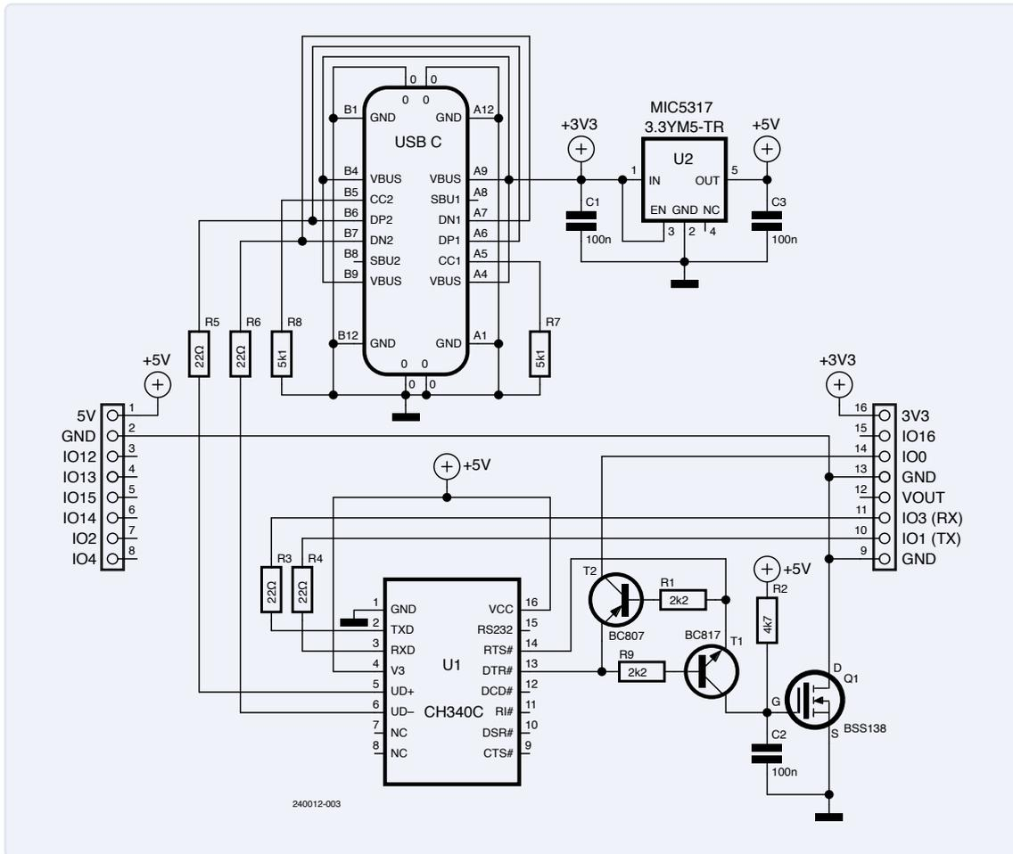
Figure 1: ESP32-CAM programmer schematic.
