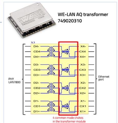
Figure 5: WE-LAN AQ transformer for galvanic isolation between PHY and Ethernet network.
