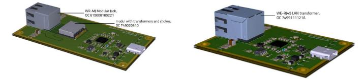
Figure 2: Gigabit Ethernet USB adapter board in the discrete version V1.0: The module with the transformers and common mode chokes is placed next to the RJ45 jack.
