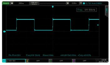
Figure 3: ESP32-C3-DevKit-M1 generating its maximum frequency while running code compiled by the Arduino framework.
