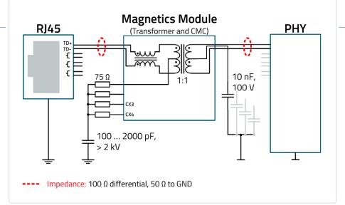
Figure 1: Schematic circuit of a 1 Gbit Ethernet interface. Only one of four channels is shown in the picture. (Source of all images: Würth Elektronik eiSos)
