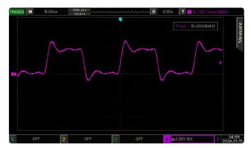
Figure 4: ESP32-C3-DevKit-M1 producing its maximum frequency while running code compiled by ESP-IDF.
