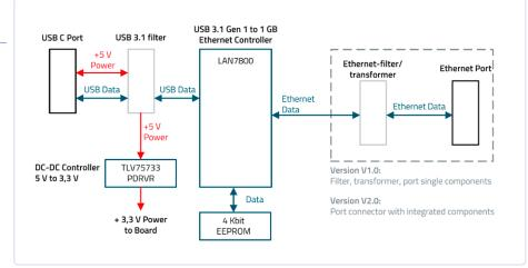
Figure 4: Block diagram of the Gbit-Ethernet-USB adapter board in both versions.
