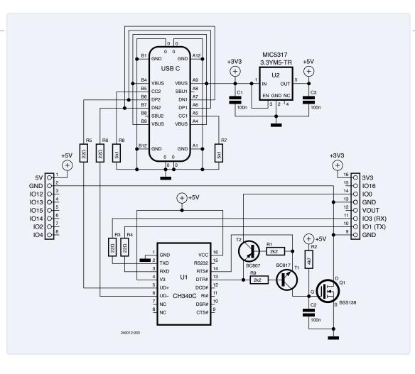
Figure 1: ESP32-CAM programmer schematic.
