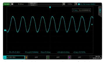
Figure 5: Raspberry Pi Pico W at 62.5 MHz using a PWM function in MicroPython.
