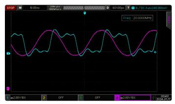
Figure 2: Comparison of square waves between the ESP32-S2 (Blue) and the UNI-T UTG962E (Pink).
