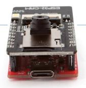
Figure 4: The ESP32-CAM should be inserted in such a way that the socket for the SD card and the USB connector are on the same side.
