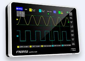
The FNIRSI 1013D is a fully featured 2-channel tablet oscilloscope with a high-resolution 7-inch LCD screen (800 x 480 pixels). The oscilloscope has a real-time sampling rate of 1 GSa/s and an analog bandwidth of 100 MHz.
