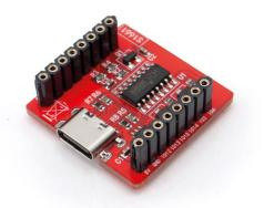
Figure 2: The board hosts the ESP32-CAM using two female headers.
