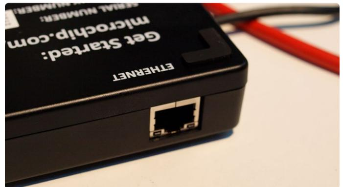
Figure 1: This port also provides Power over Ethernet capability.
