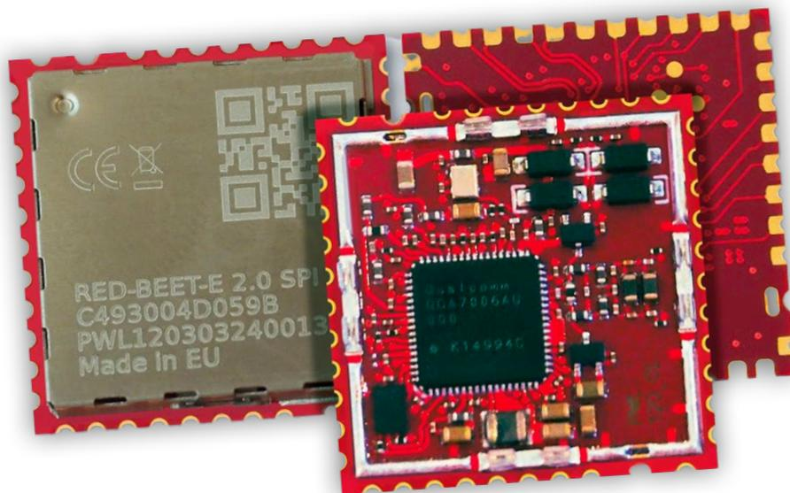
Figure 1: RED-BEET-E 2.0 for electric vehicle supply equipment (EVSE).
