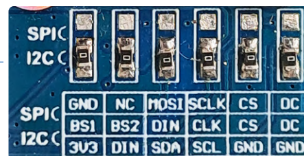
Figure 7: Detail of the display board, showing the correct position of the 0 \Omega jumper resistors for selecting the I 2 C bus.
