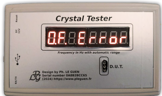
Figure 8: When the display reports "0F. Error" (Overflow error), the quartz's frequency is too high to being measured correctly.
