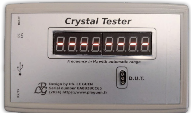
Figure 7: Dashes on the display may indicate that the quartz under test is missing, defective, or oscillating at a frequency that's too low for the measurement.
