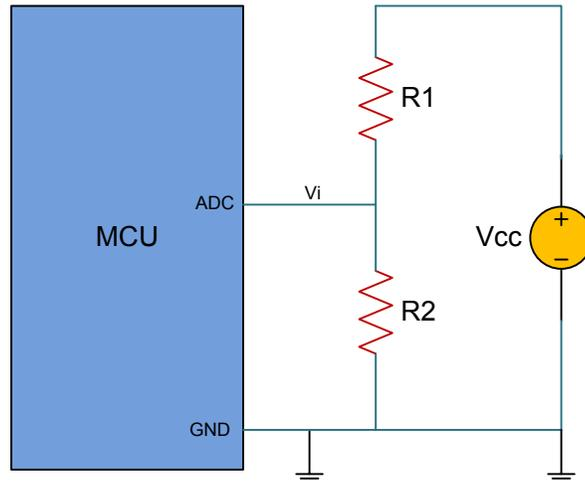
Once  $V_{IN}$  is determined, the  $V_{CC}$  can be calculated by the formula:
