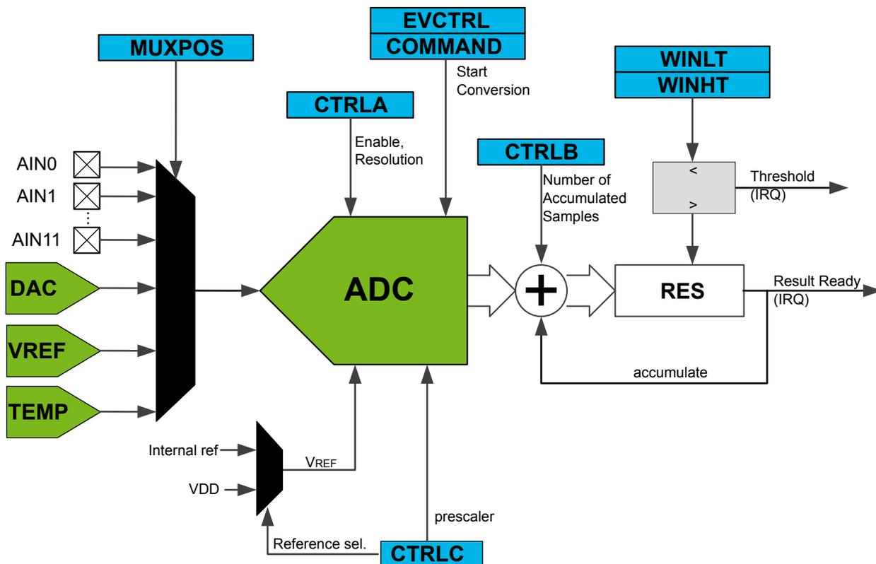
The ADC contains a sample-and-hold circuit, which ensures that the input voltage to the ADC is held at a constant level during conversion.
